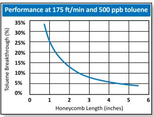
The graph above shows VOC removal using 500 ppb toluene at 175 ft/min. Toluene is a good indicator of VOCs with a vapor pressure <26 mmHg.
